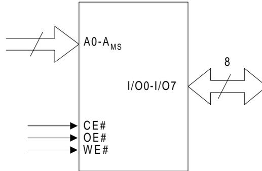
**Note:** A<sub>MS</sub> is the most significant address where A<sub>MS</sub> = A16 for Pm39F010, A17 for Pm39F020, and A18 for Pm39F040.
